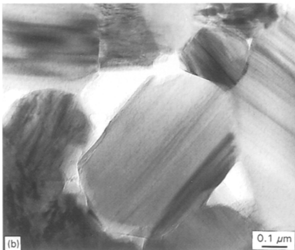
Figure 18 Transmission electron micrograph of shock-densified 7 \mu\text{m} SiC after 1950 ^{\circ}\text{C} HIPing.
