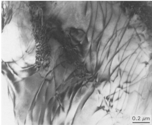
Figure 14 Transmission electron micrograph of shock-densified 7 \mu\text{m} SiC + Si + C after 1600 °C HIPing showing high dislocation densities within carbon grains.
